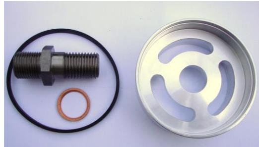
Remove the old seal which sits in the groove in the filter head. Replace with the new seal supplied in the kit. Place the alloy adaptor plate in position in the filter head and insert the hollow locating bolt (we recommend Loctite) and copper washer. Tighten the bolt using a 1" AF socket. You are now ready to fit a spin-on filter.
